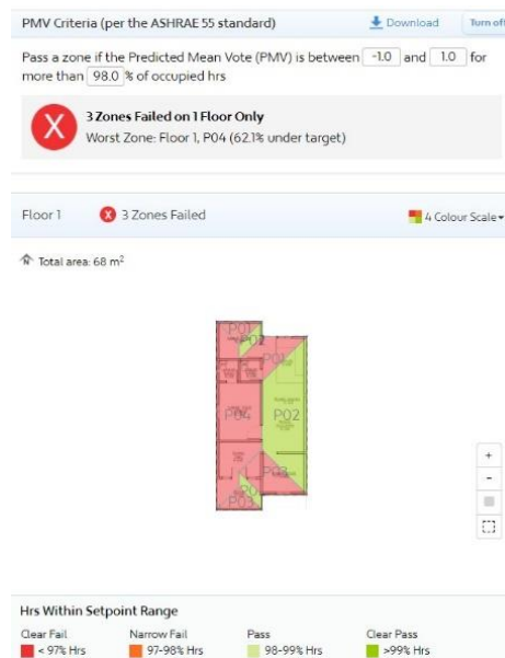
Figure 8: Results of Analysis of Thermal Comfort Conditions for Sample 2-North Houses Using Sefaira
