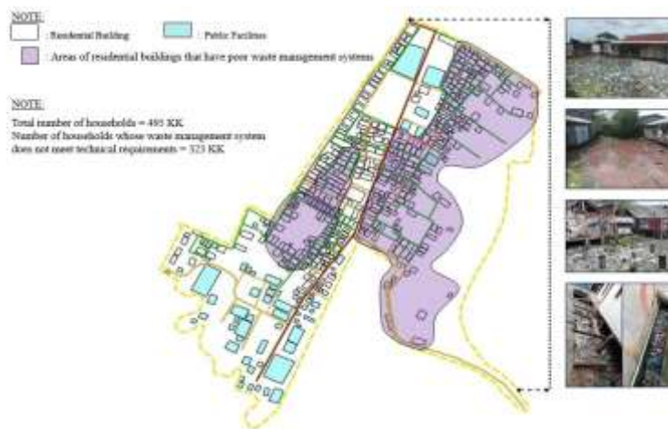
Figure 6: Condition of Waste Management System in Dusun Pasi
