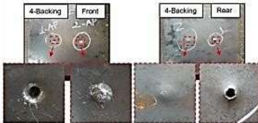
Figure 4.2.5 Rear view of the HB 550 double plate 6.2 mm thick after being hit by 7.62 AP[18]
