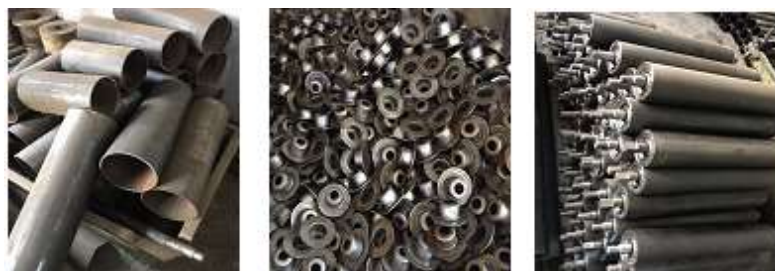
Figure 6. Steel tube, bearing cup and conveyor roller
